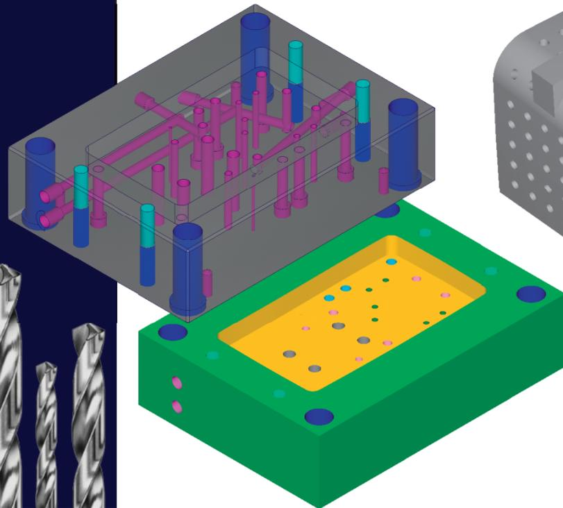
Manufacturing mold plates or machining drill forms on 5 axis parts requires many different drilling operations and optimized toolplane machining. ProDrill automates the drilling tasks of the various form types of the plates and optimizes the machining on multiple planes.
